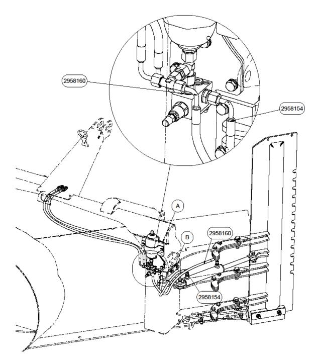
A: The bracket and plate for the accumulator must be mounted as shown in the illustration.
